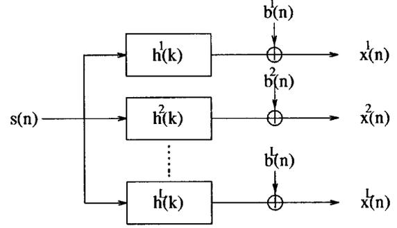
Fig. 1. Equivalent SIMO model with  $L$  channels.
