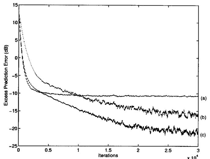
Fig. 6. Performance in the white noise case. Constraint:  $\gamma = 3$ . (a) Noisy prediction. (b) Denoised prediction. (c) Noiseless prediction.
