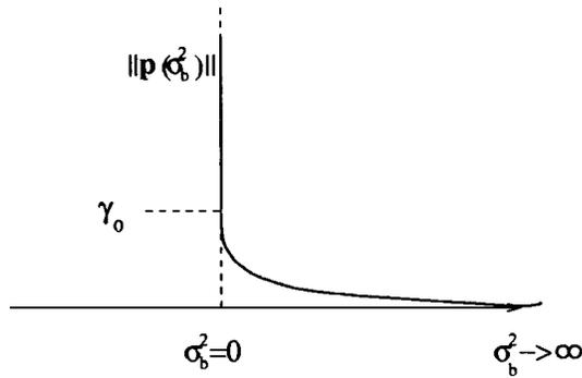
Fig. 2.  $\|\mathbf{p}(\sigma_b^2)\|$  as a function of parameter  $\sigma_b^2 > 0$ , where  $\mathbf{p}(\sigma_b^2) = (R_{sig} + \sigma_b^2 I)^{-1} \mathbf{a}$ . The norm is monotonously decreasing as the noise level increases.
