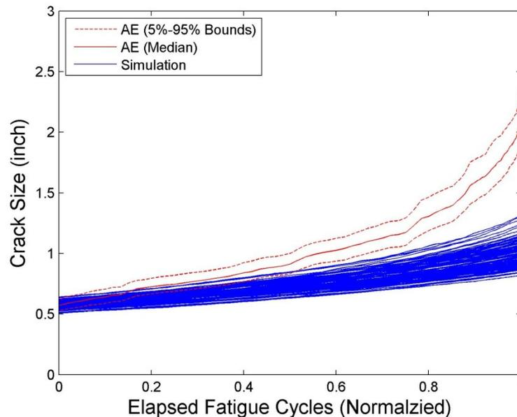
**Figure 1** Crack size prediction based on Simulation and AE NDI results
